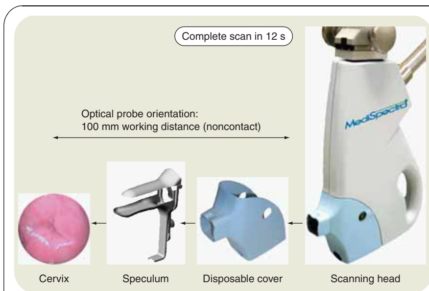
Figure 1. Scanning head is part of the LUMA™ console. Disposable covers fit within the speculum at a distance of 100 mm from the cervix and a scan is obtained.
